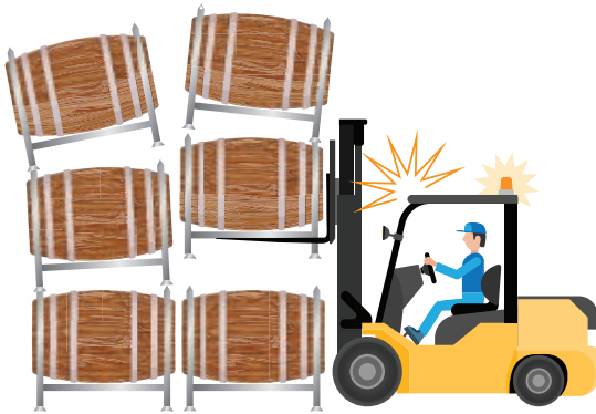
Competitor Locating feet that protrude can cause dangerous catch of adjacent stacks
